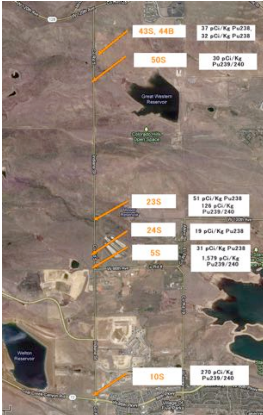
Figure 7: Locations and concentrations of plutonium detections in Kaltofen's 2011 study. Note that 1,579 pCi/kg at Indiana Street and 96 th Avenue represents 81x background radiation.
